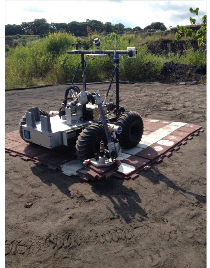
Assembling a launch/landing pad. Credit: PISCES
